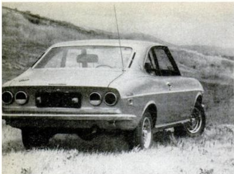
RX-2 COUPE spans 97-in. wheelbase, R-100 uses 89-in. Radial tires and sporty wheels both are standard
